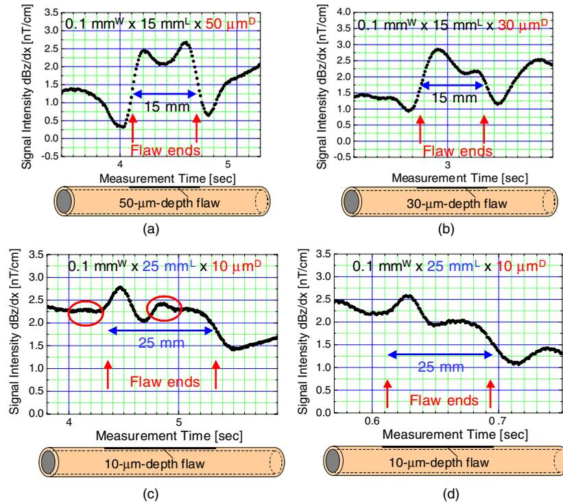
**Figure 3.** Measurement results on (a) 50  $\mu\text{m}$ -depth flaw, (b) 30  $\mu\text{m}$ -depth flaw, (c) 10  $\mu\text{m}$ -depth flaw and (d) 10  $\mu\text{m}$ -depth flaw. In the measurement on (d), the specimen was moved at 32  $\text{m min}^{-1}$ , while in the other cases ((a)–(c)) the specimens were moved at 1.6  $\text{m min}^{-1}$ . The circles in (c) indicate the noises that may be caused by the vibration of the tube being moved slowly.
