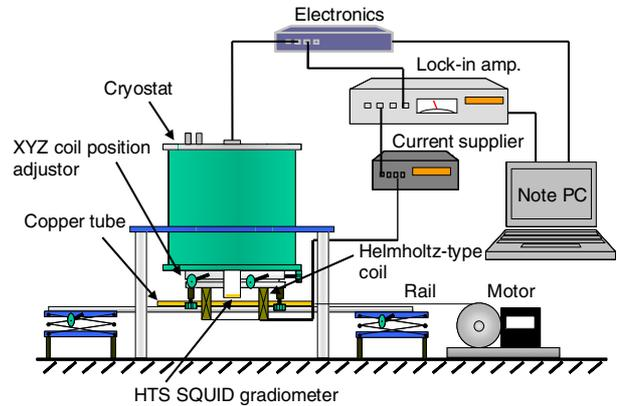
**Figure 2.** Schematic diagram of the SQUID NDE system.
