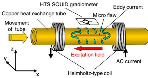
**Figure 1.** Principle of the SQUID NDE for a copper tube.
